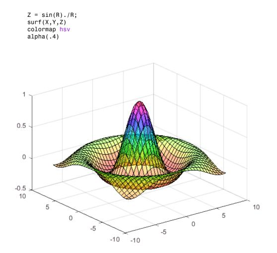
MATLAB displays a surface with a face alpha value of 0.4. Alpha values range from 0 (completely transparent) to 1 (not transparent).
