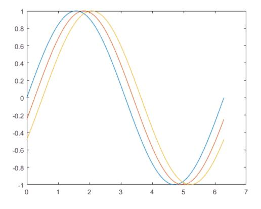
The legend function provides an easy way to identify the individual lines: legend(' $\sin(x)$ ', ' $\sin(x-.25)$ ', ' $\sin(x-.5)$ ')
