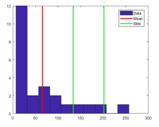
The plot shows that some of the data are more than two standard deviations above the mean. If you identify these data as errors (not features), replace them with NaN values as follows:
