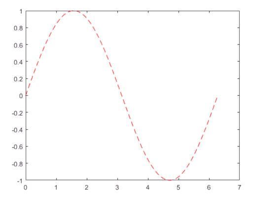
The 'r--' string is a *line specification*. Each specification can include characters for the line color, style, and marker. A marker is a symbol that appears at each plotted data point, such as a +, 0, or \*. For example, 'g:\*' requests a dotted green line with \* markers.
